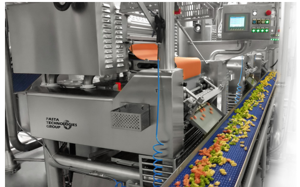
TRICOLOR CAPPELLETTI LINE, 1000 KG/H.
