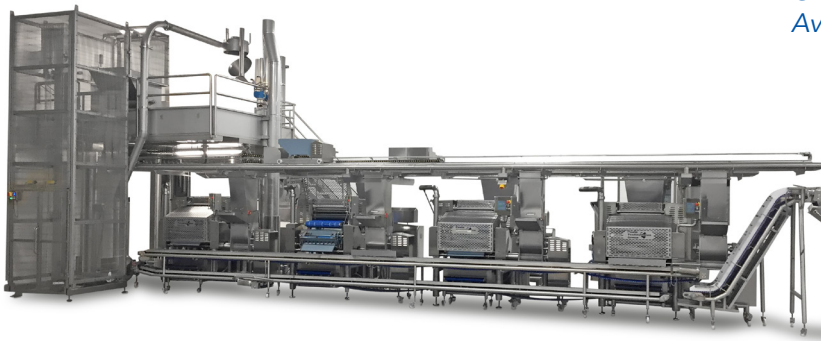
TORTELLONI LINE, 2000 KG/H WITH AUTOMATIC DOUGH AND FILLING DISTRIBUTION SYSTEM.
