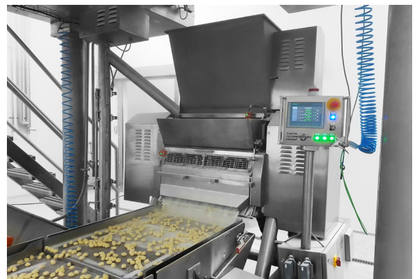
GNOCCHI LINE MOD. GN24, 1500 KG/H. Available in several sizes.
