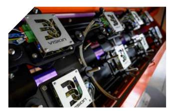
**High resolution multispectral cameras SWIR (1024 pixel), up to 4 wavelengths.** These cameras allow unreachable results until now, **recognising polymers**, selecting shells and **foreign bodies in dried fruits** and where there are chemical differences even if not visible by human eyes.
